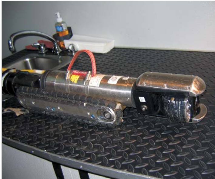
The OZII crawler camera relays video of pipeline inspection to CUES Granite XP software, where crews can record data to be later entered into a GIS map.
