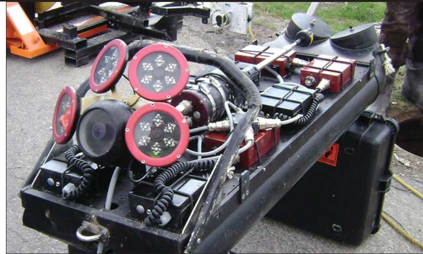
The Fly Eye system from CUES, shown ready for insertion. The system can be deployed through a standard manhole.
