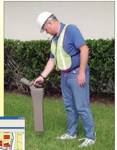
Granite XP Wireless GPS Mapping Stick from CUES Inc.
