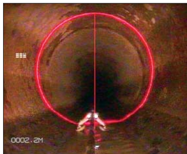
A ring of laser light is shown inside a pipe free of roundness defects.
